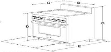
NOTE: 24" (61 cm) minimum clearance between the cooktop and the bottom of the cabinet when the bottom of wood or metal cabinet is protected by not less than 1/4" (0.64 cm) flame retardant millboard covered with not less than No. 28 MSG sheet metal, 0.015" (0.4 mm) stainless steel, 0.024" (0.6 mm) aluminum, or 0.020"
