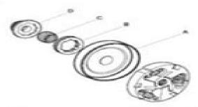
Unbolt and remove the clutch drum (A), chain sprocket (B), needle bearing (C) and pump drive wheel (D).
