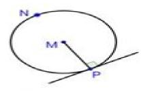
A radius is perpendicular to a tangent at the point of tangency.
