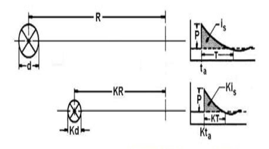
Figure 2.4: Geometric representation of Hopkinson-Cranz blast wave scaling [1].
