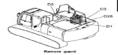
(2) Release internal pressure of tank. Remove cap on air breather and push valve (head of bolt) by your finger.
