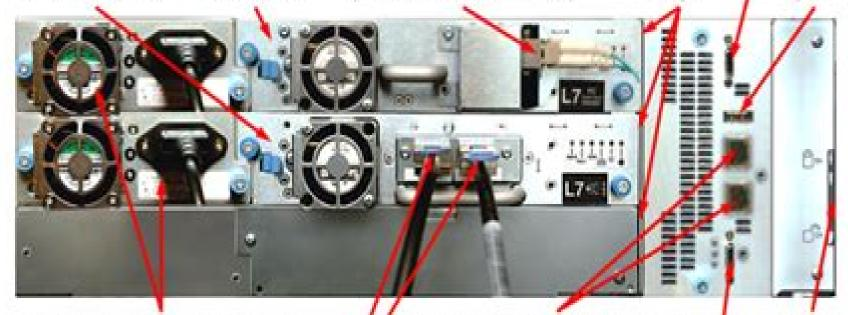
Up to 2x redundant hot-swap power supplies (IEC 320-C14 AC power connector) 2x 10/100/1000 Mb Ethernet management ports (RJ-45) Module alignment mechanism
