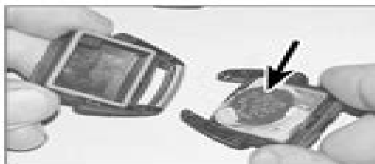
23.1b . . . and remove the circular battery
