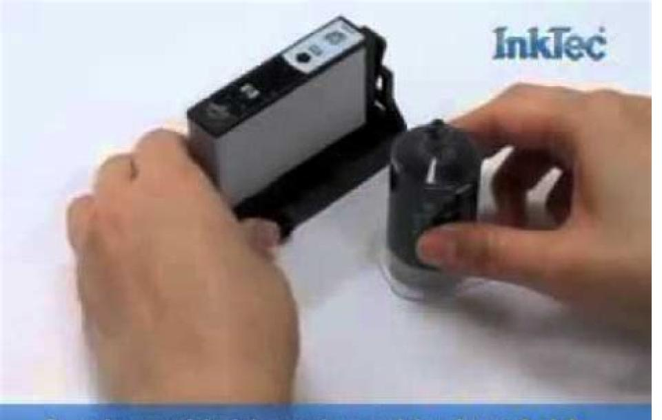
Open the cap of the ink container, and then insert the ink container deep into the ink injection inlet which is the lower part of the refill clip.
