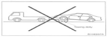
Do not tow vehicle with rear wheels raised under any circumstances since this will damage bumper.
