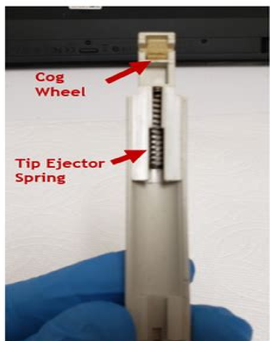
Tip Ejector Pusher Mechanism w/ Cog Wheel and Spring
