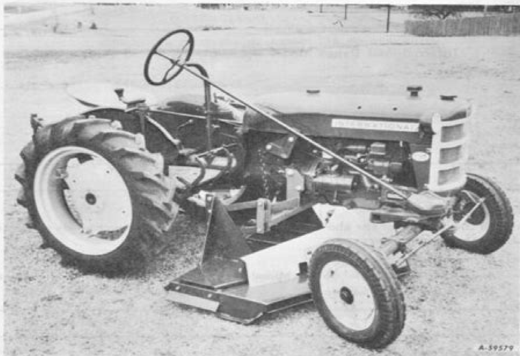
International Danco Model C-1 Rotary Mower mounted on the International Cub® Lo-Boy® Tractor.
