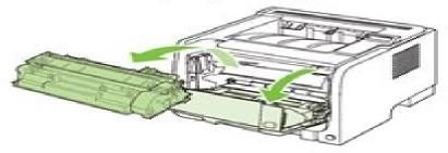
Remove the new print cartridge from the bag. Place the used print cartridge in the bag for recycling.
