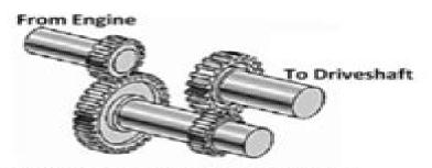
The Cluster (Counter) Gear Enables the Output to Spin The Same Way as the Input.
