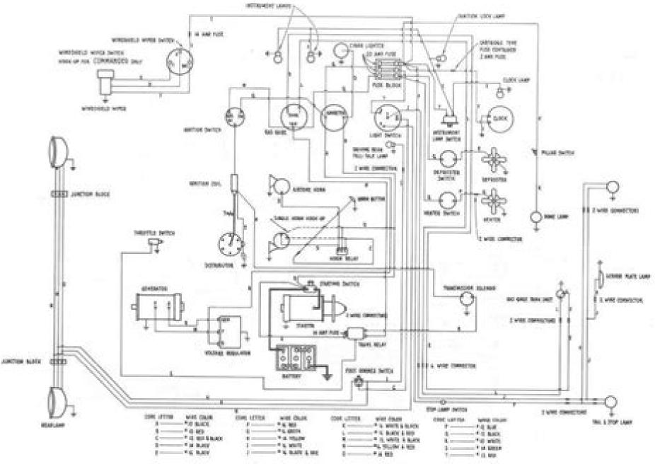
CHAMPION AND COMMANDER Wiring diagram of the electrical system used in the Champion and Commander models.
