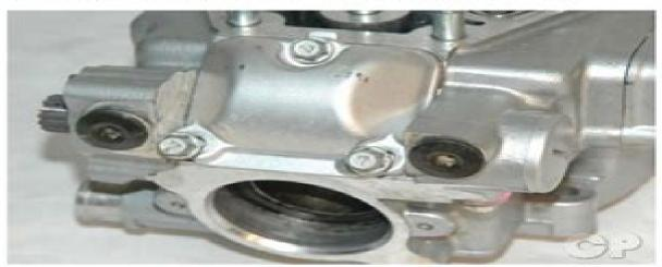
Remove the three bolts that secure the KIPS cover in place with an 8 mm socket.
