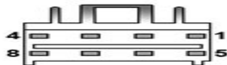
8 pin GM 89047379 (19115652) amplifier wiring harness connector
