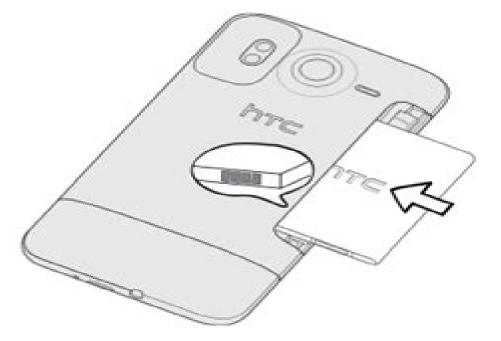
4. Put back the battery compartment cover, pushing the battery all the way in.
