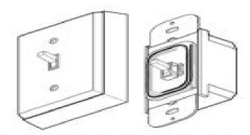
You'll need to buy a 9-volt alkaline battery for the wireless switch. In typical use, this battery will last one year.
