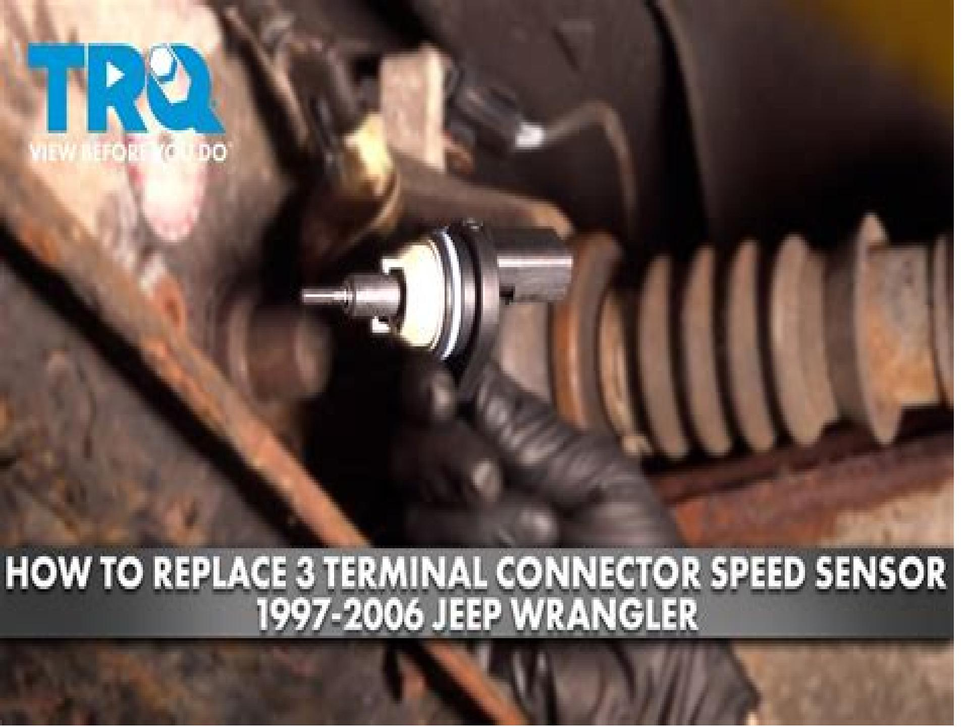
**HOW TO REPLACE 3 TERMINAL CONNECTOR SPEED SENSOR
