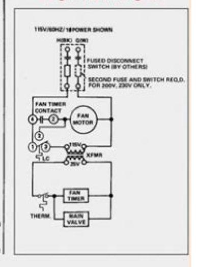
\*ALTERNATE XFMR. PRIMARY XMFR. WIRES 230V /60HZ/1# - BK & Y 200V /60HZ/1# - BK & R TAPE OR WIREAUT
