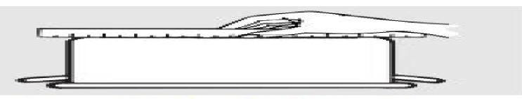
Check pans for flat bottoms by using a straight edge.
