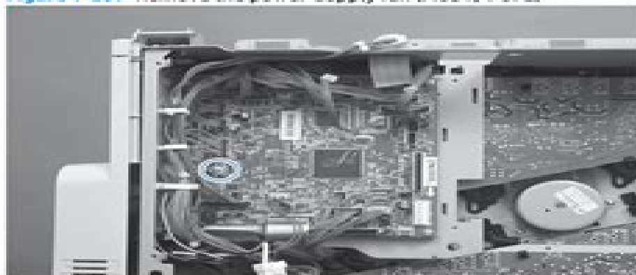
Figure 1-297 Remove the power-supply fan (M651; 1 of 2)
