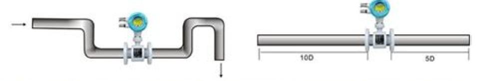
Install in a U trap to ensure meter body is always completely full of liquid, Allow 10 diameters of straight pipe before the meter & 5 diameters after to develop a smooth flow profile through the meter. More specific requirements are shown below
