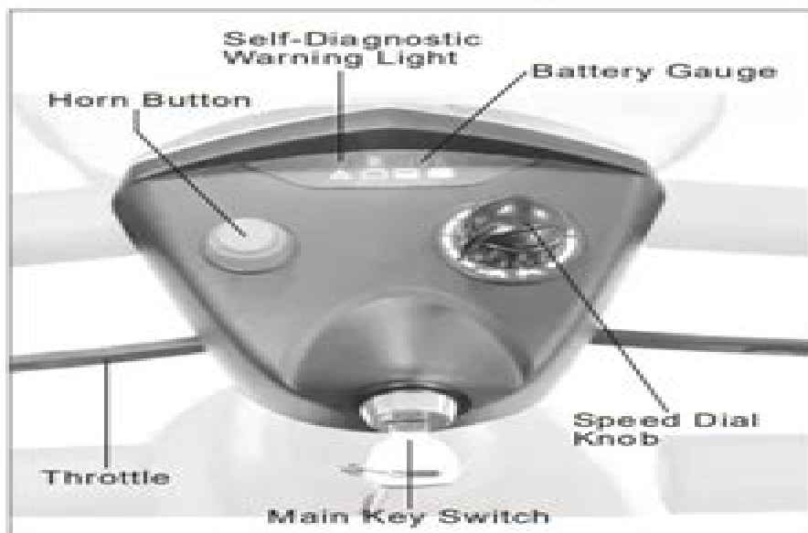
Figure 2 - EW-M39 Top Control Panel
