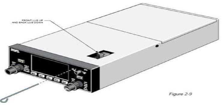
Insert the KLN 90B insertion/removal tool (supplied with unit) in the small hole located on the right side of the front of the unit (figure 2-9). A standard 3/32 inch Allen wrench may also be used.
