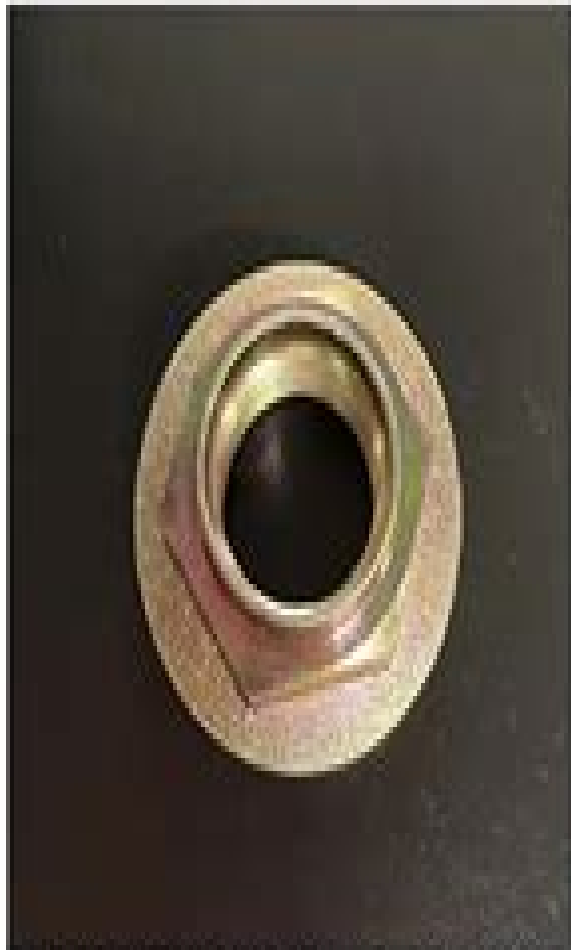
USE A NEW NUT OR COTTER PIN
