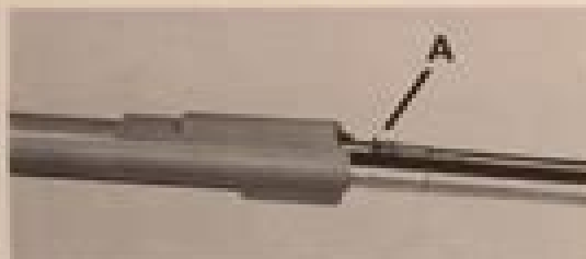
2. To complete assembly, insert the lower wand, large end first, into sheath from the bottom until the latch (A) engages.
