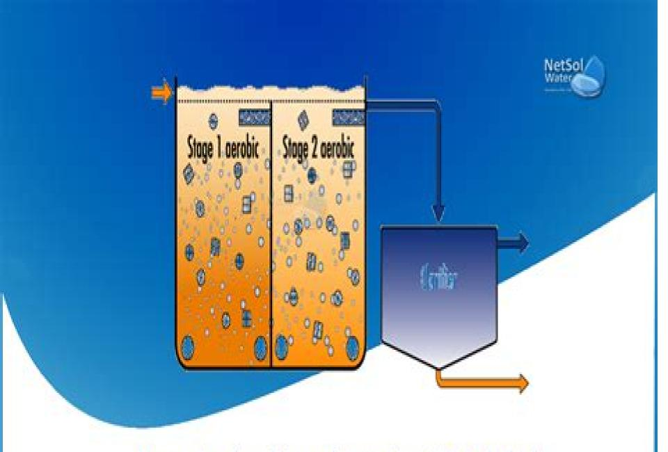
How to Design, Size and Capacity of MBBR Tank
