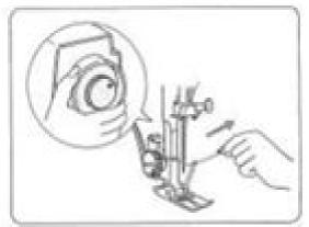
Turn the balance wheel slowly towards you with your right hand until the reedle goes down and continue turning belance wheel until the take-up lever is at its highest position. Lightly draw up the needle thread forming a loop of the bobbin thread.
