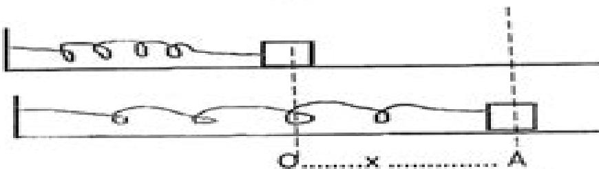
If an external force  $F_{\text{ext}}$  displaces the body from position O to A through displacement  $x$  then By Hook's Law
