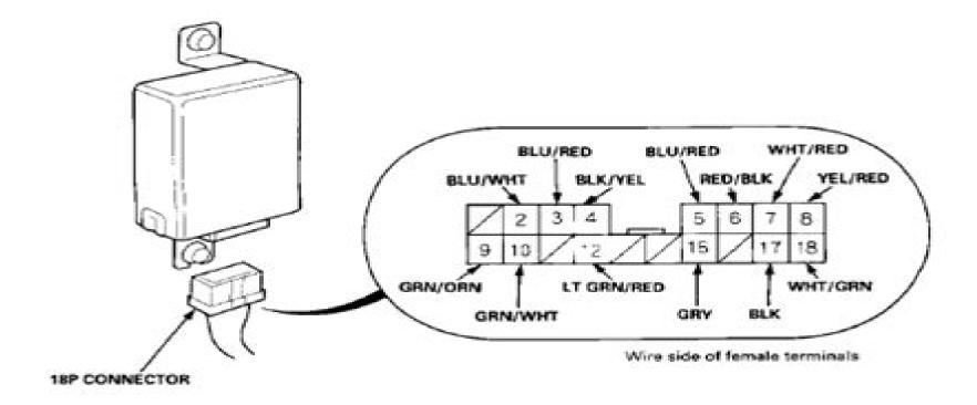
Disconnect the 18P connector from the power door lock control unit.
