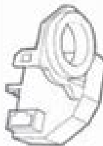
Immobilizer-keyless control unit (Built-in receiver)
