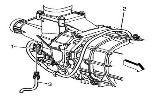
Fig. 22: View Of HO2S Electrical Connector Courtesy of GENERAL MOTORS CORP.
