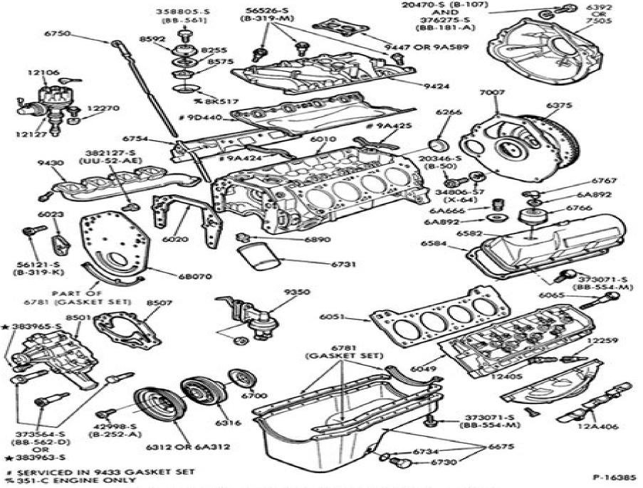
CYLINDER BLOCK and RELATED PARTS (EXTERNAL) — TYPICAL 1980/82 8 CYL. 351M (5.8L) and 400 (6.6L)
