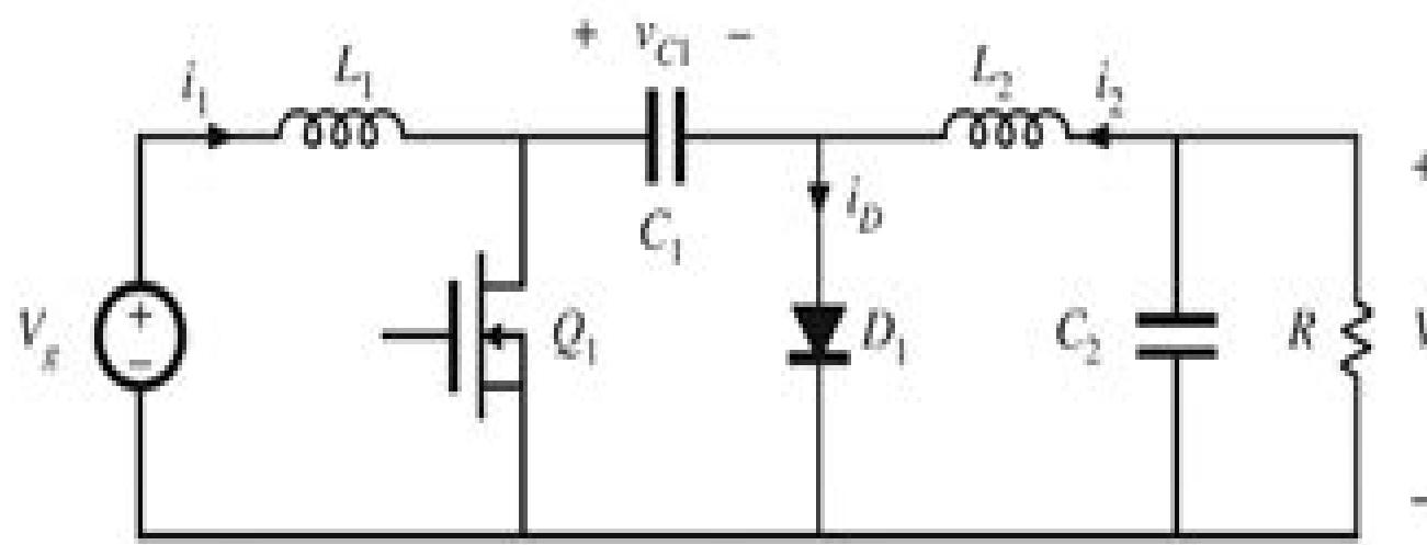
Fig. 5.24 Ćuk converter. Problems 5.7, 5.8, 5.14, and 5.15
