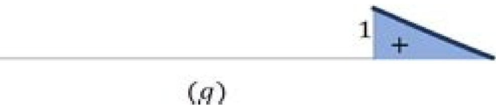
Influence line for shear V_c at hinge C
