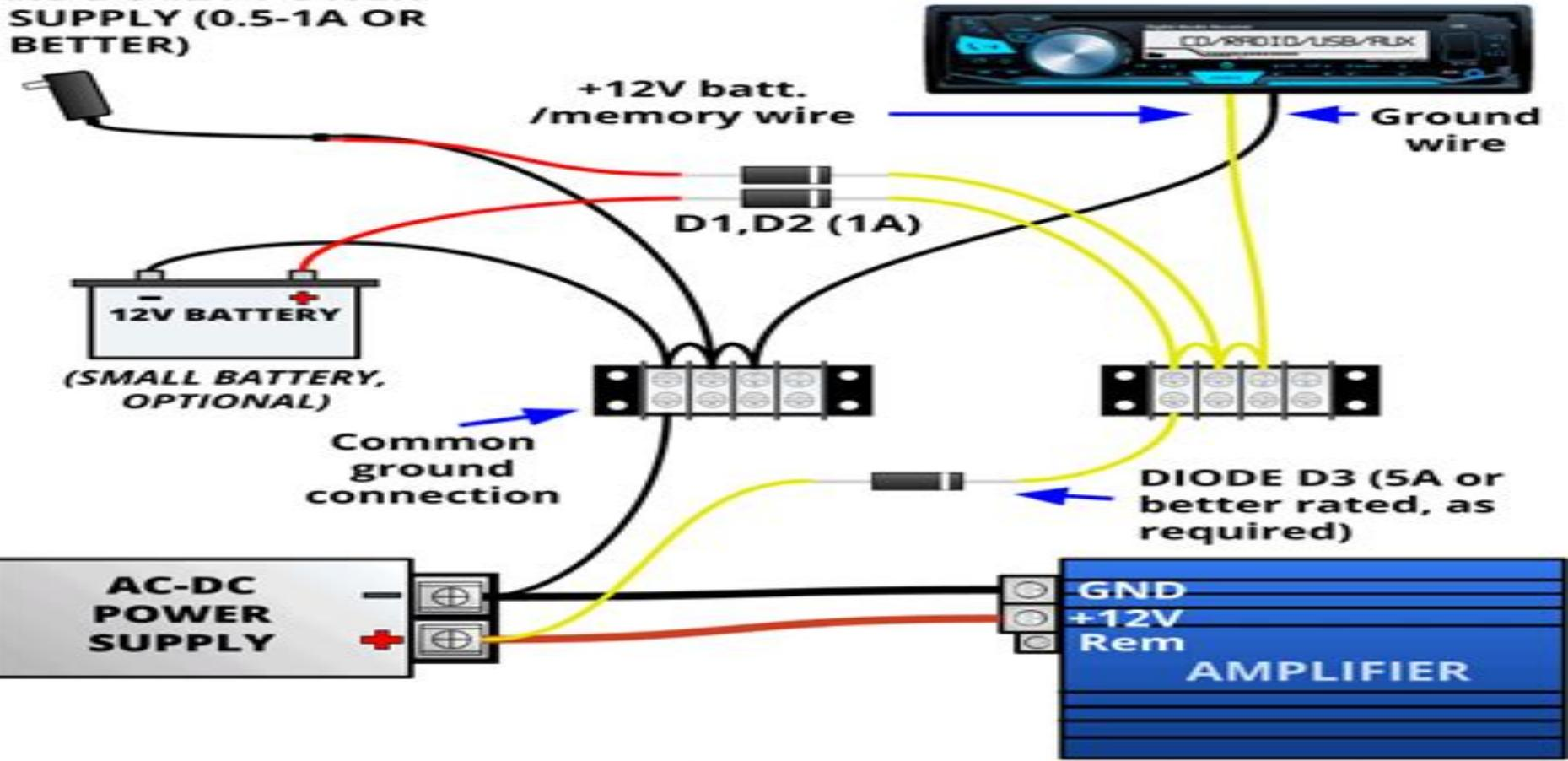
**\*\*Diode D3 supplies power to the head unit when switched on therefore should be rated for the head unit's maximum current draw. Optionally, you can also use multiple diodes in parallel instead of a single diode of higher current rating if they add up to the same or more.**
