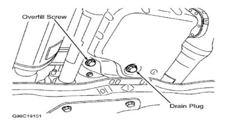
Fig. 3: Identifying Drain Plug & Overfill Screw (4L30-E) Courtesy of ISUZU MOTOR CO.
