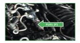
Remove the female connector attached to the fuel sensor and attach this to the male connector on the TDI-Tuning harness. Once this has been attached, you should use the other connector to attach it to your vehicles connector.
