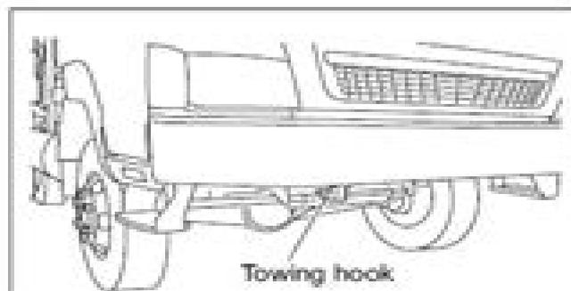
1. Tow the stranded vehicle using a vehicle whose gross weight is equal to that of the stranded vehicle (14,050 lbs., 6,375 kg). Attach the rope or wire rope to the towing hook of the towing vehicle.
