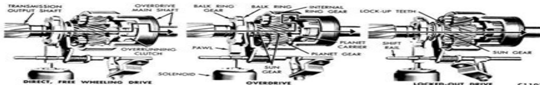
FIG. 6—Overdrive Power Flow
