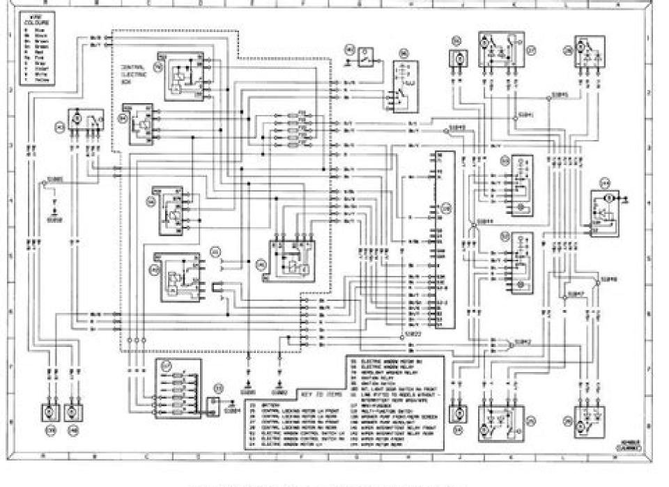
Diagram 12: Typical wash/wipe, central locking and electric windows
