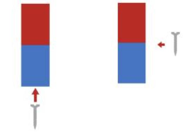
Fig 1. Magnetic Field Strength and Distance. An iron nail is attracted to a magnet as iron is a magnetic material. The magnetic field is strongest at the poles. An object placed close to the pole will experience stronger attraction than if it is placed to the side.
