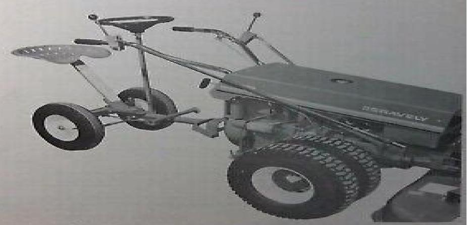
The Steering Sulky is for use with the Two Wheel tractor
