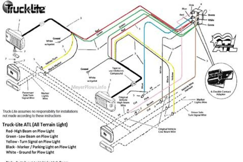
Pink - Switch out to Vehicle High Beam Brown - Switch out to Vehicle Low Beam Blue - Switch input from Vehicle High Beam wire White - Switch input from Vehicle Low Beam wire
