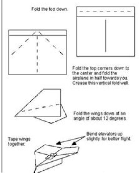
For best flight. Bend the leading edges of the wings down at a slight angle, fold the back half of the wingtips up, and make sure you add just a little up elevator. The wings should be perpendicular to the fuselage. When throwing the plane, hold it in the center of the fuselage and throwill at an angle upwards. (However, even if you throw it fairly level, it will refuse to make a short flight!)
