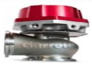
G arrett Vent | External Wastegates regulate turbocharger shaft speed by venting exhaust gas around the turbine stage of the turbocharger. CFD optimized design maximizes flow and delivers optimum boost control. Advanced thermal optimization increases durability of the diaphragm. The cap design makes spring changes and serviceability of the entire GVW lineup easier and more reliable to perform.
