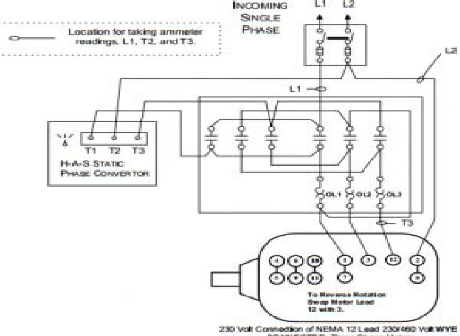
30 Volt Connection of NEMA 12 Lead 230/460 Volt WYE CONNECTED. Three Phase Motor (Use with 230 Volt H-A-S Static)
