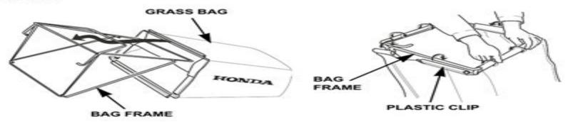
Lift the the discharge guard and install the grass bag.
