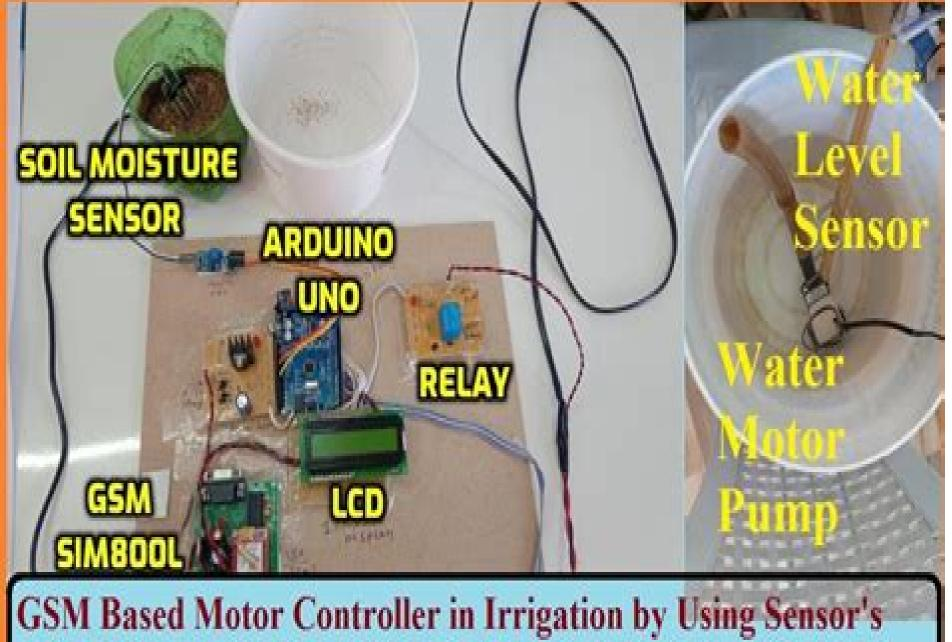
GSM Based Motor Controller in Irrigation by Using Sensor's Soil Moisture + Tank Water Level
